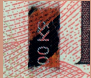
Pole Feature – hatching with lighter and darker rhomboids – appears on security windowed thread when Pole Tester is applied
