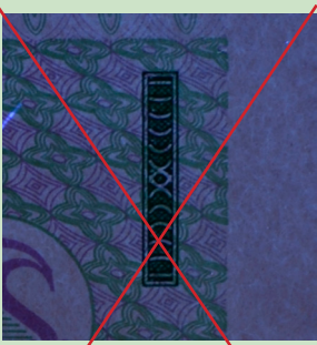
blind code does not fluoresce
