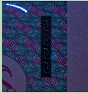
blind code does not fluoresce
