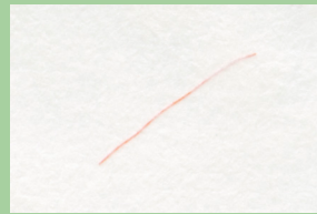
orange protective fibres spread randomly across entire paper surface
